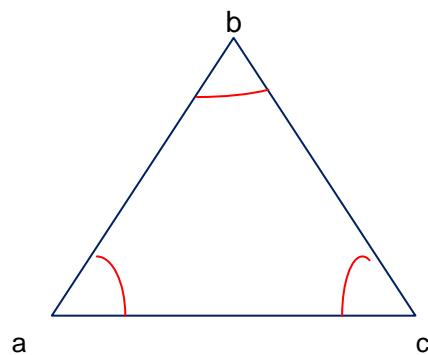
$$\overline{bc}^2 = \overline{ab}^2 + \overline{ac}^2 - 2 \cdot \overline{ab} \cdot \overline{ac} \cdot \cos \hat{a}$$
